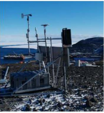
Our BEL-v50 is a compact, silent and lightweight vertical axis turbine. Designed to trickle charge your batteries or provide energy for low power electronic devices such as data-logging or telemetry equipment.
